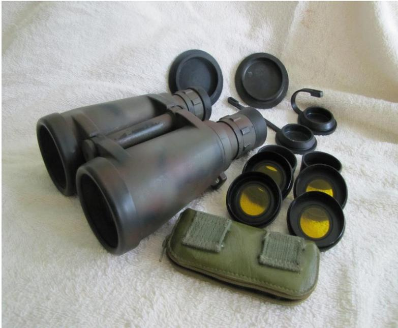
**Fig. 4. ELCAN 7X50 binos with all the issued gear: yellow filters, eyepiece caps, objective caps, extra pair of eye cups, and a small, green neck strap case for the yellow filters. The green neck strap is missing.**
