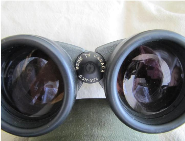
**Fig. 8. ELCAN 7X50B, civilian version, with the “MADE IN CANADA” disc. Serial # 0176 indicates that this was # 176 of about 400 issued, and # C 317 is ELCAN’s optical computing number.**
