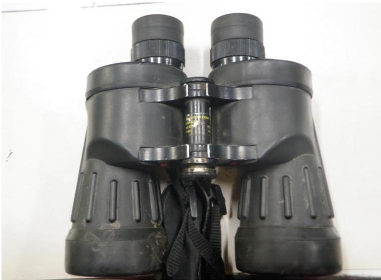
**Fig. 9. Fujinon 7X50 Porro-prism Type 1, black rubber armored bino, the first of two kinds Fujinon bins serving the Canadian Forces since about 1999-2000. (Photo by W. O. Geoff Closs, 1PPCLI, Edmonton.)**
