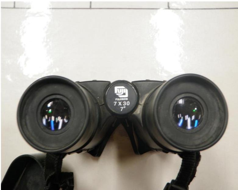
**Fig. 10. Fujinon 7X30 roof-prism, black rubber armored bino, the second of two kinds of Fujinon bins serving the Canadian Forces since about 1999-2000. (Photo by W.O. Geoff Closs, 1PPCLI, Edmonton.)**
