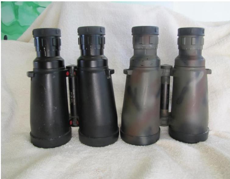
**Fig. 3. Two ELCAN 7X50 binos. The black one (left) is as factory issued (obvious red Nitrogen purge screws). The camo-colored version was painted by the user, and the red purging screws were painted over.**
